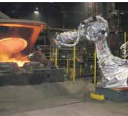
Robots can be used to improve worker safety and energy efficiency on the melt floor. 9
