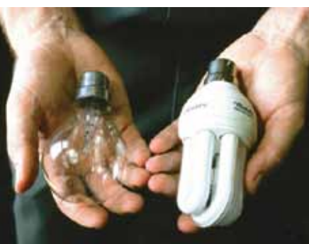
Light bulbs with an efficiency of less than 15 lumens per watt such as incandescent light bulbs are being phased out.
