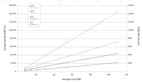
The Compressed Air Energy Calculator is a free internet based calculator that determines the potential savings that can be made by checking and repairing leaks, reducing air pressure or lowering the inlet air temperature. For more information visit: www.aircompressors.com/ educational-resources/energy-calculator
