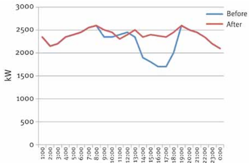
Figure 5: Production delay due to blown fuse
