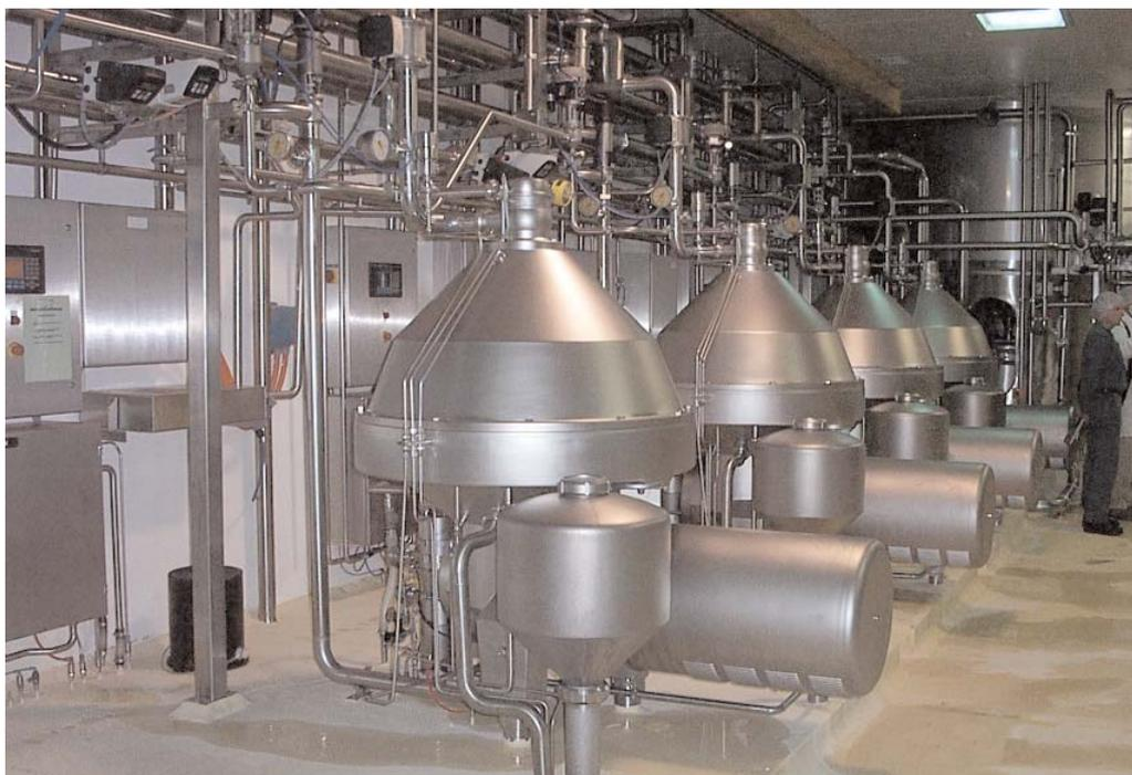
*Optimising de-sludge frequency for all processes that utilise centrifugal separation of liquid milk streams will ensure that losses of milk components are minimised.*
