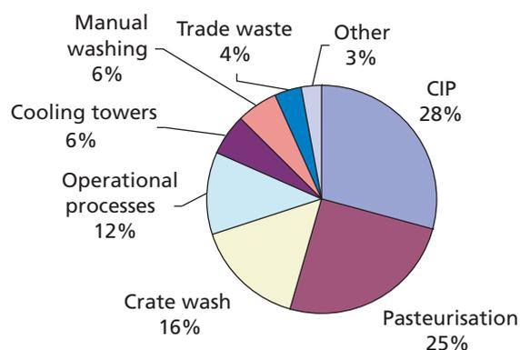
Many dairy processors track the overall consumption of water by monitoring the ratio of water to raw milk intake. Water consumption in Europe has been reported to range from 0.2 to 11 L/L milk (Daufin et al. 2001) with effluent volumes per raw milk intake in the same range. Ratios for Australian processors producing any combination of white milk, cheese, powders or yoghurts range from 0.07 to 2.90 L/L milk, with the average being around 1.5 L/L milk (UNEP 2004).
