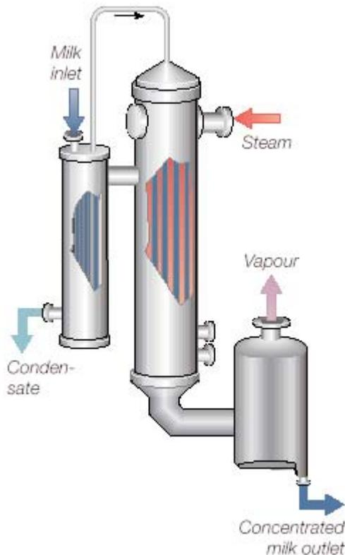
**Figure 4.3** Single-effect falling film evaporator schematic
