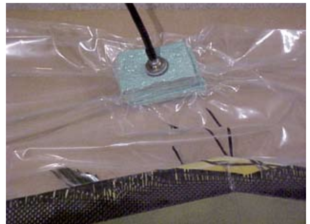
A vacuum bagged mould
