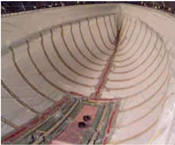
A hull set up for infusion moulding
