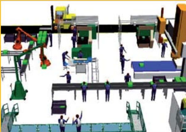
Digital manufacturing allows for virtual simulation of [2] workflow arrangements and avoids costly setup mistakes
