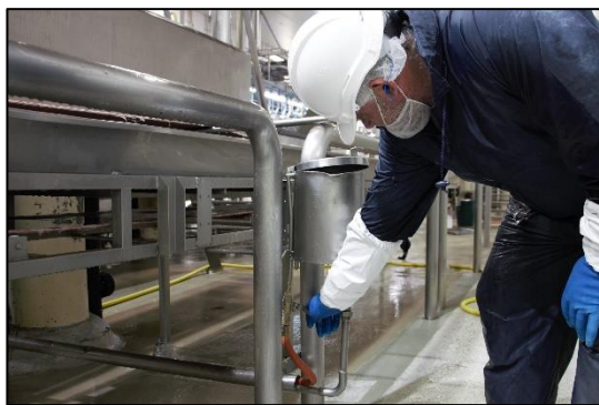
Turning off continuous flow knife steriliser with shut off valve at the end of operations.
