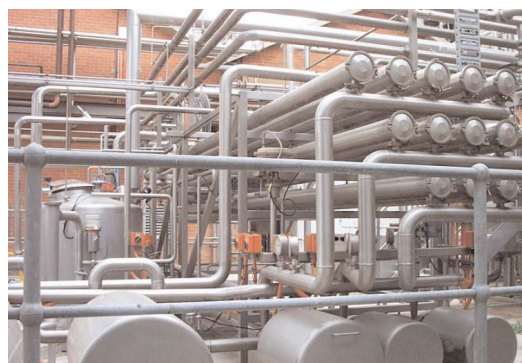
A major advantage of membrane separation technology is that the separated substances can be recovered in a chemically unchanged form.
