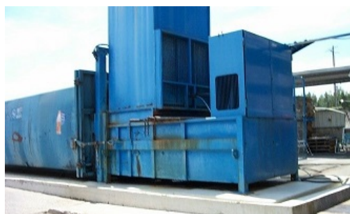
Compacting solid waste can help reduce transport costs and save on storage space
